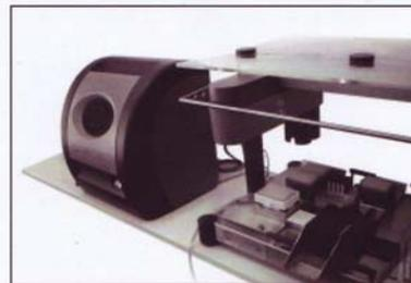
The UltraPlex SmartReader and SmartStation equipment used to perform and analyse assay and profile tests
